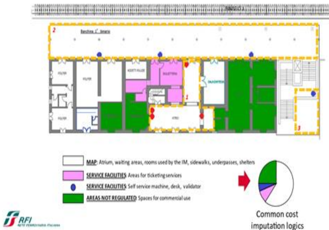
Figure 10. Types of service facilities in a station
